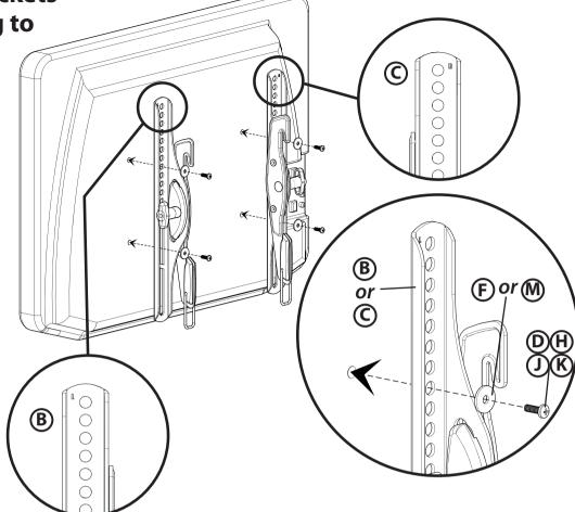
**Option 2: Attaching to a curved or** irregular mounting surface
